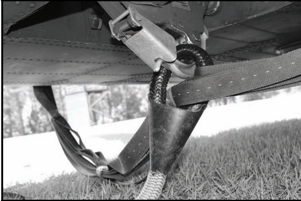
Figure 5-3. SPIES rope rigging on UH-60
